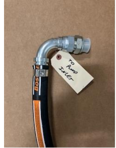
Fig. 8: Install 90° radius hose to pump inlet.
