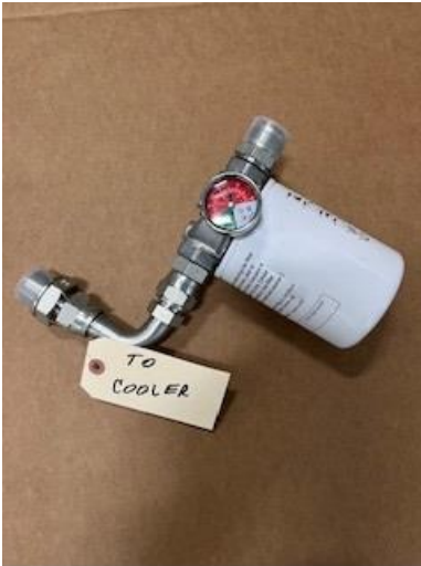
Fig. 6: Install 90° radius filter head to heat exchanger.
